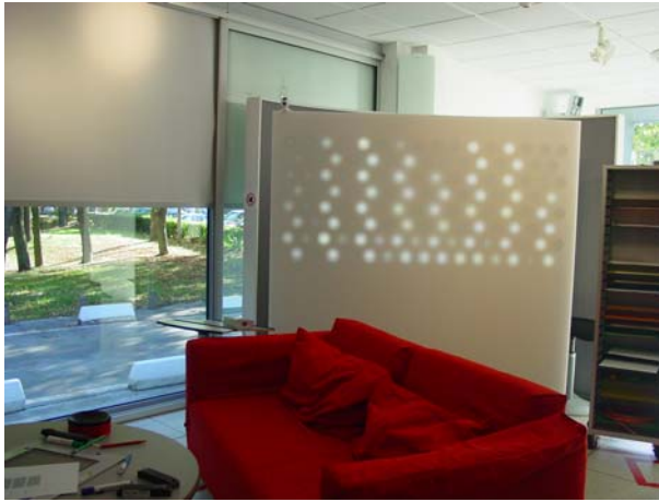
Fig. 2. The Hello.Wall – an ambient display communicating awareness information between different locations via a range of dynamic light patterns
